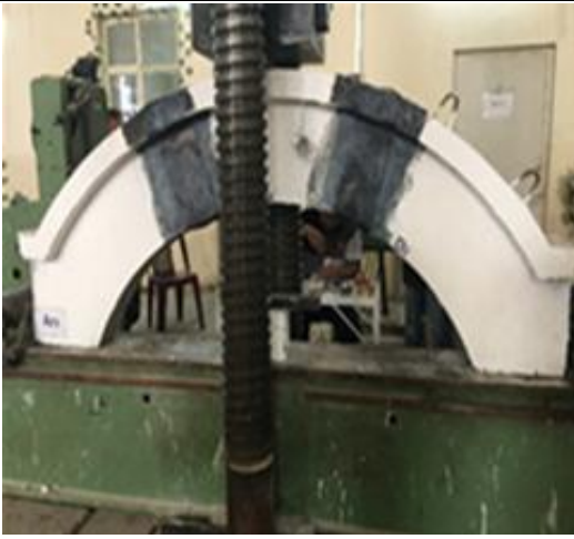
Figure 4: Specimen AR9 before and after test with cracks propagations
