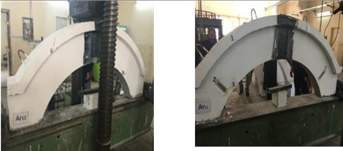
Figure 7: Specimen AR12 before and after test with cracks propagations
