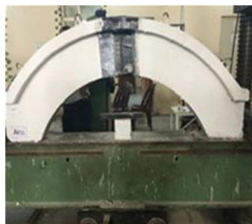
Figure 6: Specimen AR11 before and after test with cracks propagations
