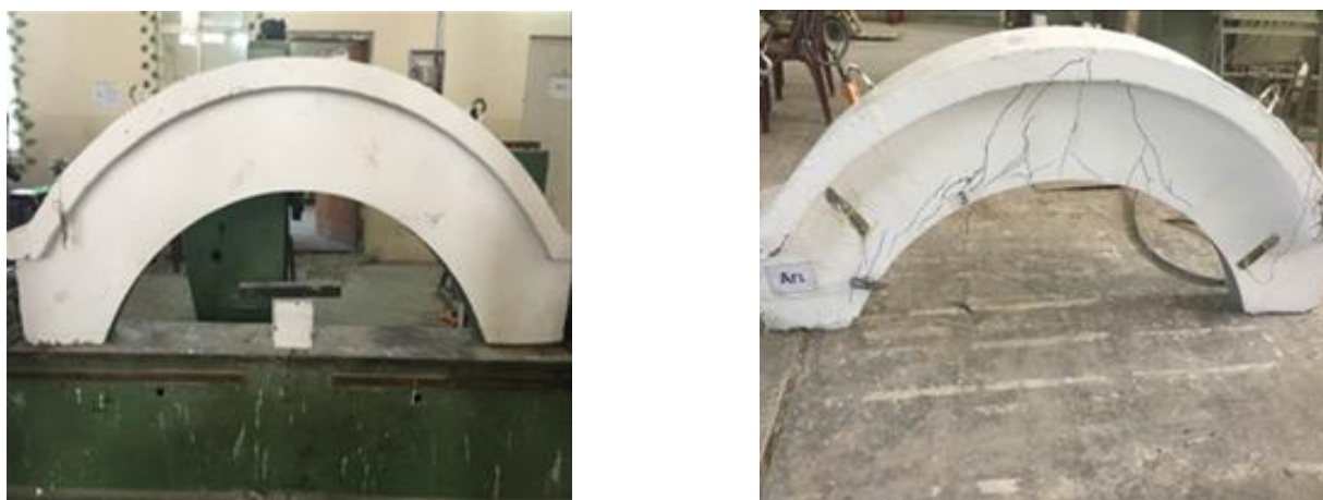
Figure 3: Specimen AR1 before and after test with cracks propagations
