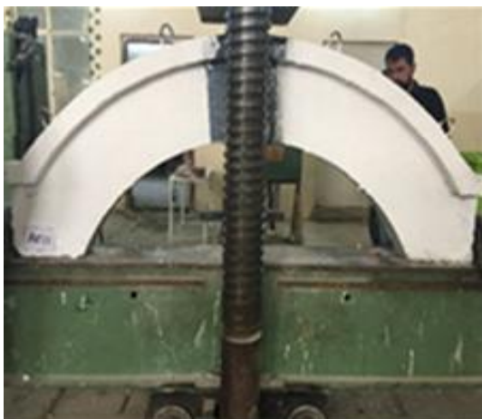
Figure 6: Specimen AR11 before and after test with cracks propagations
