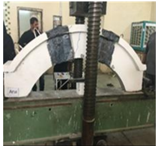
Figure 5: Specimen AR10 before and after test with cracks propagations
