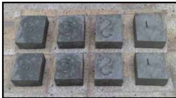
Figure 2. Concrete specimens used for testing thermal conductivity.
