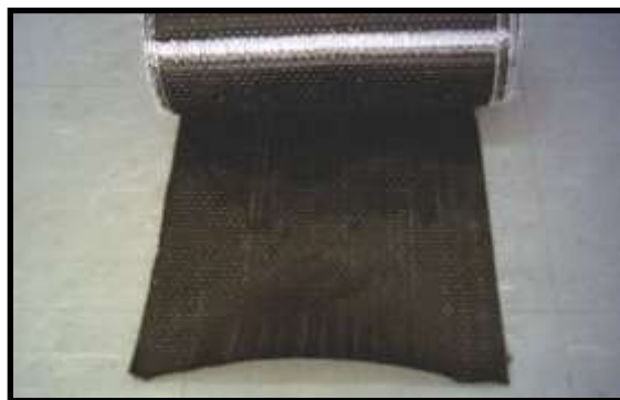
Figure 4. The CFRP mat used.
