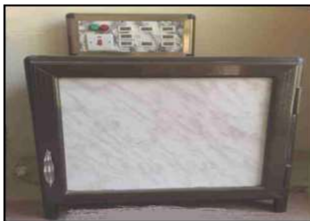
Figure 6. The device used to measure the thermal conductivity of concrete.
