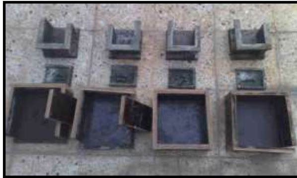
Figure 1. Wooden molds for specimens and steel molds for concrete cubes.
