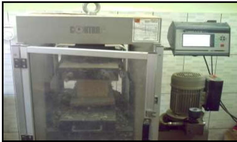
Figure 5. The device used to testing concrete compressive strength.
