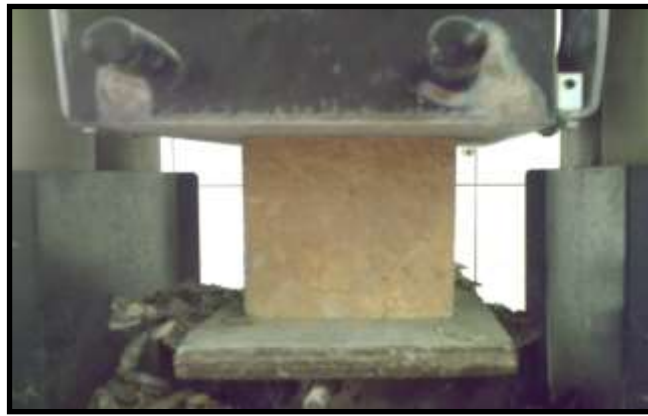
Figure 3. A standard concrete cube prepared for testing compressive strength.
