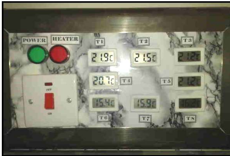
Figure 7. Details of the electronic board of the thermal conductivity measuring device.
