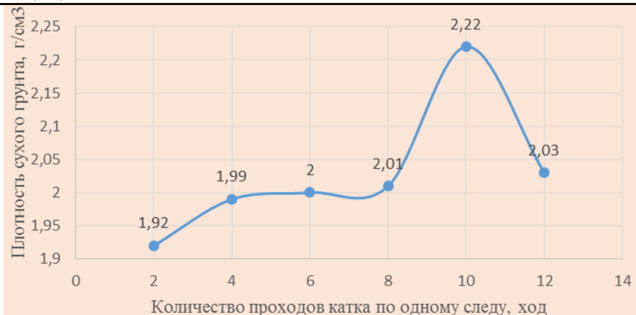
Fig.3. Graph of the dependence of the density of dry soil with a layer thickness of 80 cm on the number of passes of a smooth roller (26000 kg.) with the vibrator turned on, water irrigation 160 l / m 3 NB, stone.
