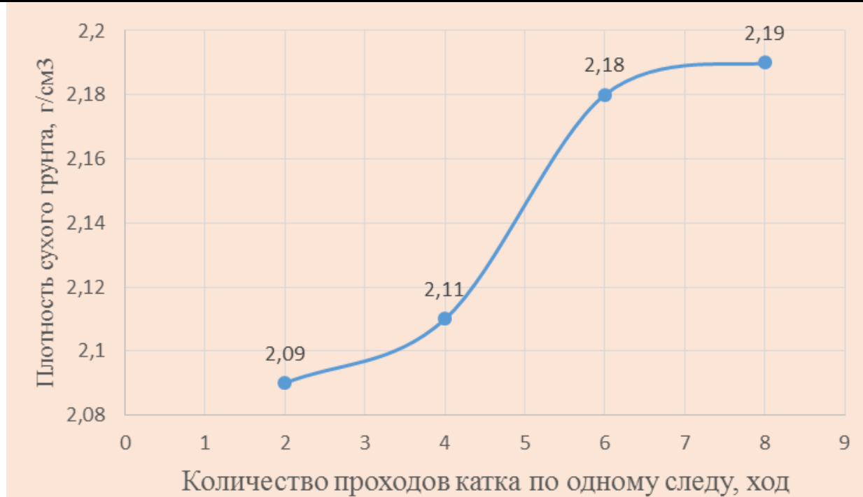
Fig.1. Graph of the dependence of the density of dry soil with a layer thickness of 50 cm on the number of passes of a smooth roller (26000 kg.) with the vibrator turned on, water irrigation 160 l / m 3 WB, stone.
