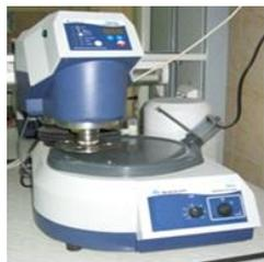
**Figure 2 - Automatic Grinding Machine Buehler Vector Head/Beta.**
