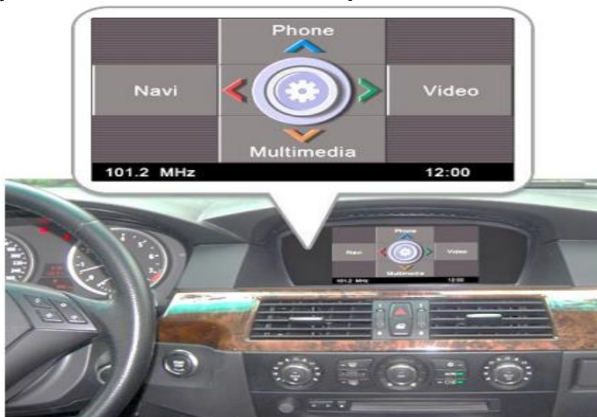
Figure 1 - On-board computer with a liquid crystal display of a BMW car (CCC system - CarCommunicationComputer)
