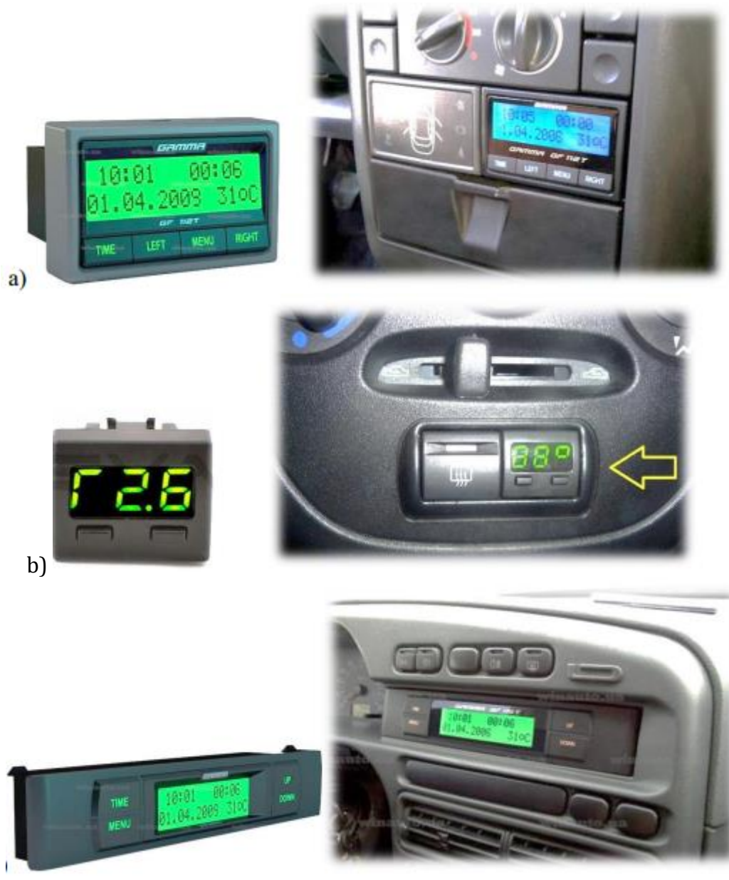
Figure 2 - Appearance of automobile trip computers of various types, Russian-made cars: a) - the standard size of the car clock; b) - button size; e) - standard size of the car radio.
