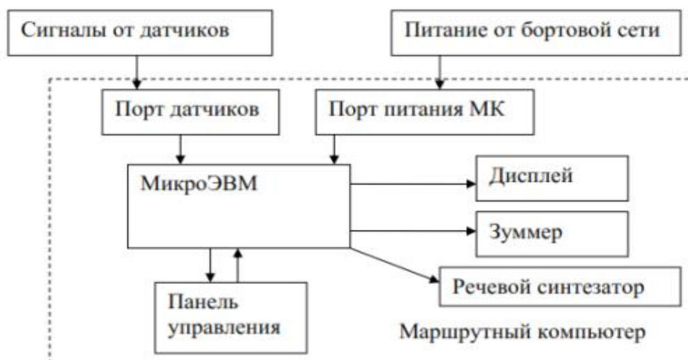
Figure 3 - Structural diagram of an automobile trip computer.
