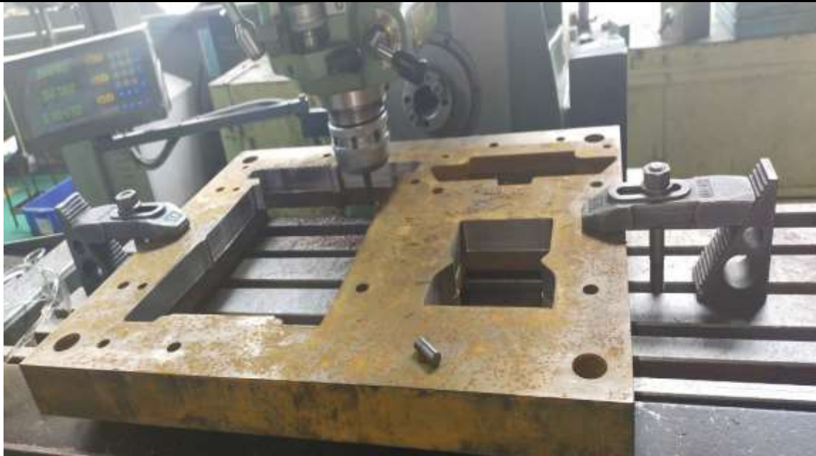
Fig 2. Restoring the contact welded matrix part to the size of the milling cutter.
