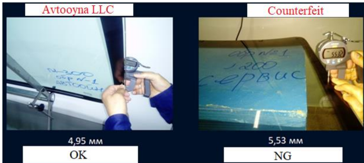
Fig. 4. Windshield thickness measurement
