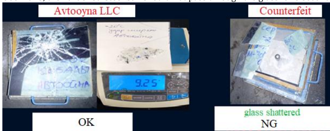
Fig.2. Small ball test.
