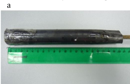
Figure. 3. Design of anchor sleeve for elongation test of composite reinforcement: a – appearance; b – device diagram
