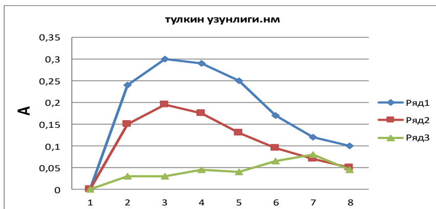
Figure 1. Absorption spectrum of 1,3,4-thiadiazole-2,5-dithiol organic reagent before (1) and after (2) immobilization, complex (3)
