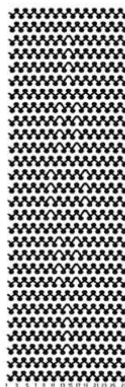
Figure 6. Option 4 - a graphical record of a press weave with an index of 4.
