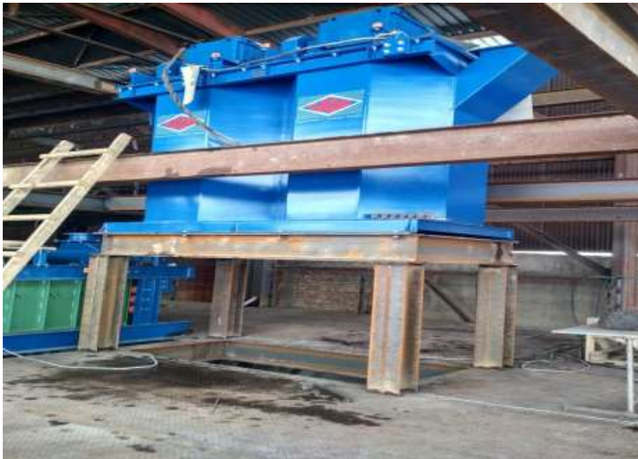
Figure 2. Scrubbers. (they allow effective disintegration of materials with a clay content of up to 50% or more.)
