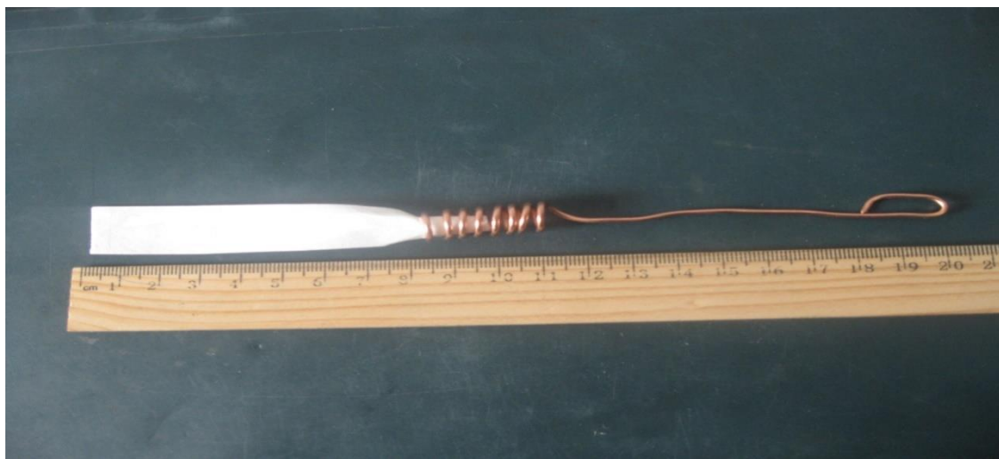
Figure 3. Placing a paper tape from a fuming acaricidal filter that holds the copper device
