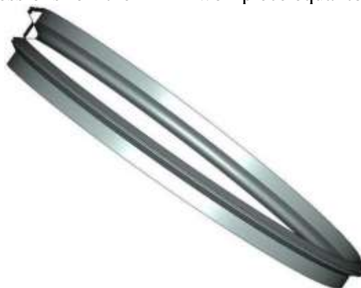
Fig.3. Determination of the diameter of the workpiece for rolling thread M 20x1.5 using 3D modeling.
