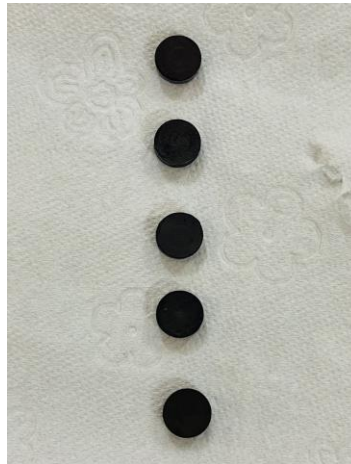
Figure (2): Transformation of powder to compact sample.
