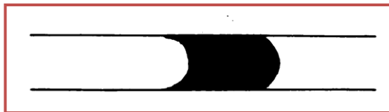
Fig. 1.8 Sample shape resulting from laminar flow with molecular diffusion
