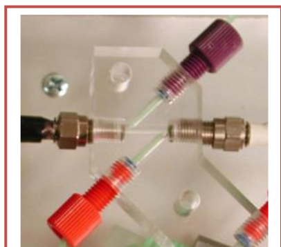
Fig. 1.19 (a) Z- flow cell with 10 mm light path (b) Z- flow cell with 10 cm light path
