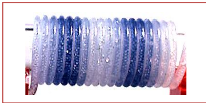
Fig. 1.26 Coil tube packed with glass beads
