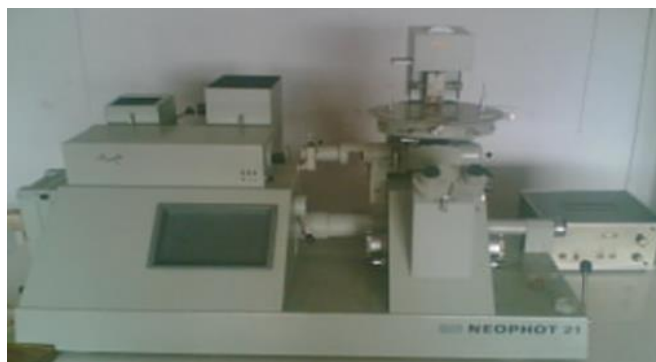
Fig. (4) Micro-hardness tester with Optical microscope
