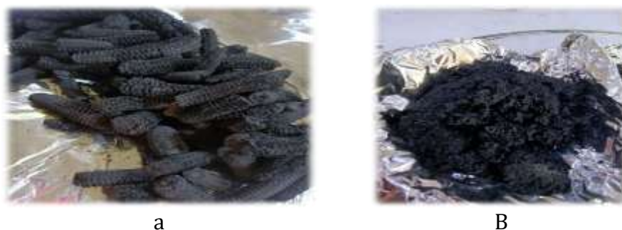
Figure 2. Corn cobs after pre-carbonized and grind /sieve.
