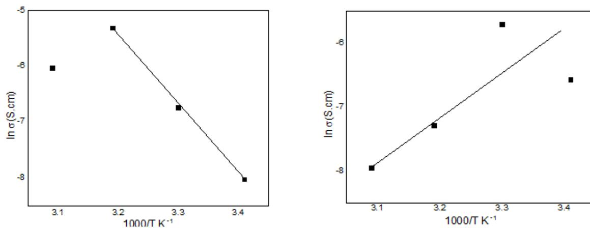
Figure (2) depicts the conductivity of films at graphene ratios of 1%, 3%,5% and 7% w/w. Figure 2. shows the relationship between 1000/T and ln σ<sub>dc</sub> for polyester/ graphene for which the activation energy E<sub>a</sub> could be estimated from the slope of the straight line using the following [19].
