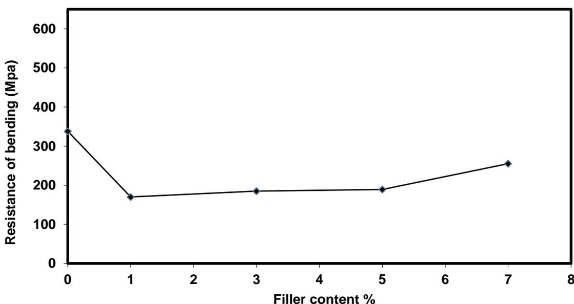
Figure ( 3 ) resistance of bending for Polyester reinforced with different percentage of graphene
