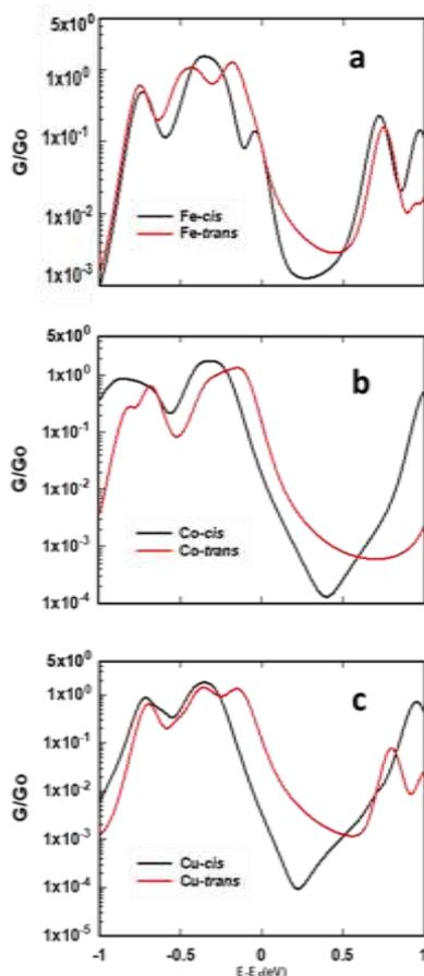
**Figure 3.** Room temperature electrical conductance of metallophthalocyanine (MPc) in *cis*, and *trans* configurations.
