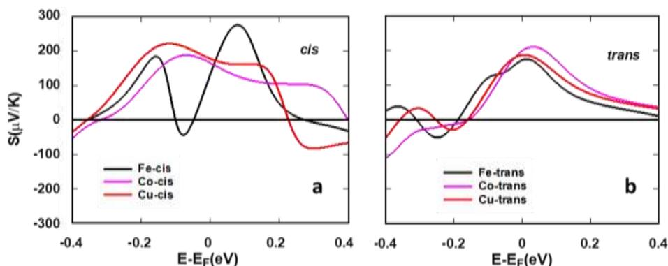
**Figure 4.** (a) Seebeck coefficient ( $S$ ) curves of metallophthalocyanine (MPc) in *cis* (b) *trans* configurations.
