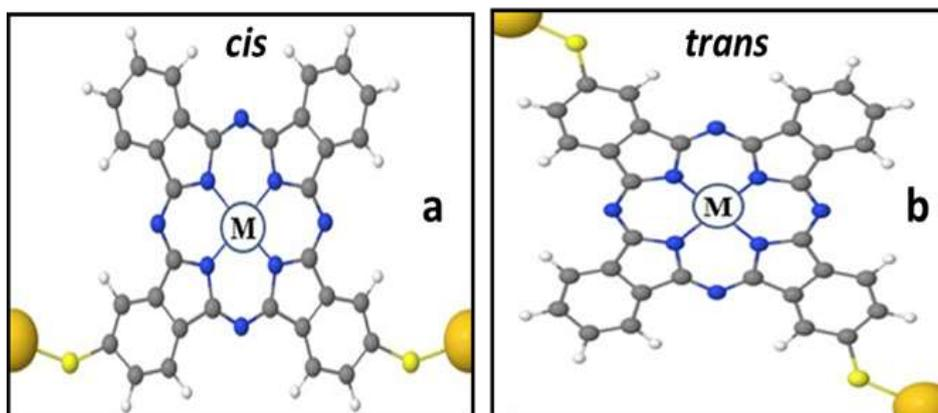
**Figure 1.** Metallophthalocyanine (M-Pc) molecule structure sandwiched between two gold electrodes in two different configurations (a) *cis*, and (b) *trans*.
