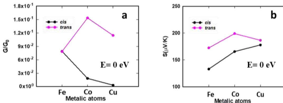
**Figure 5.** Comparison of (a) electrical conductance and (b) thermopower (S) values for all structures of metallophthalocyanine (MPC) in *cis*, and *trans* configurations.
