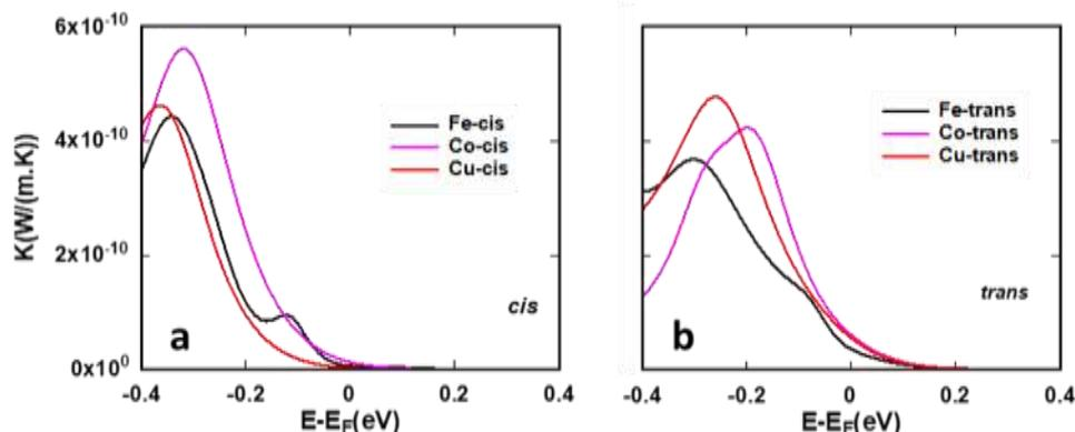
**Figure 6.** (a) Thermal conductance  $k$  as a function of energy of metallophthalocyanine (MPC) in *cis*, (b) *trans* configurations.
