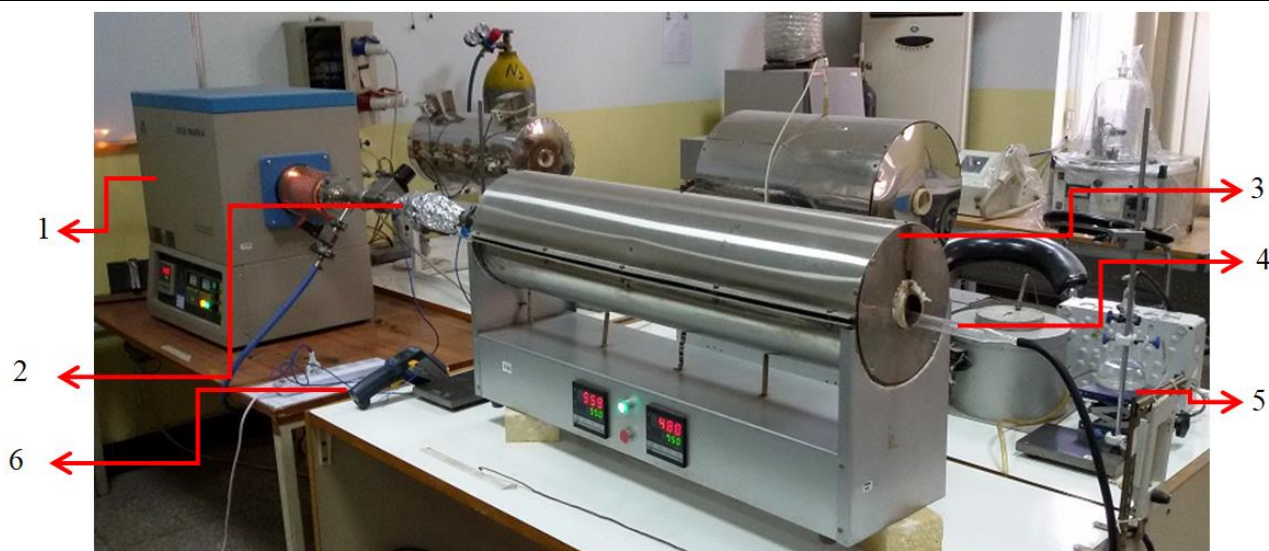
Figure 1: Coating preparation tool utilized in the current investigation: 1. Part of Evaporation, 2. Path of Ti-Based vapor, 3. sedimentations Chamber, 4. Quartz pipe for sedimentations, 5. Exhausting gas part, 6. thermometer.
