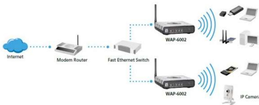
Figure 1; showing wireless access points.
