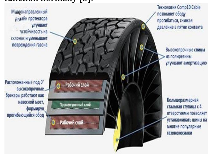
Fig.1. Elements of an airless tire:
