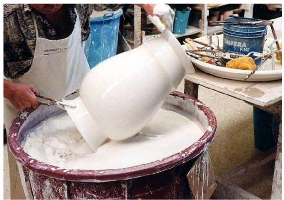
Polished white products are dried in the sun for about 20 minutes. Ceramics are fired twice. The first firing is raw and unglazed. After the first firing, a hand painting is applied with natural pigments such as copper, cobalt, iron and manganese oxides. After that, the product is once again covered with glaze and the second firing is carried out at a temperature of 1000 degrees Celsius.
