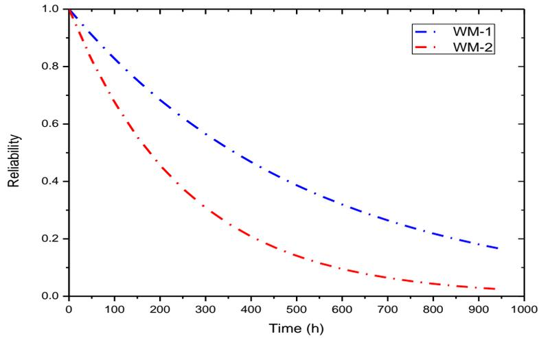
Figure 1: Comparison of reliability indicators of WM -I and WM electrical subsystems .
