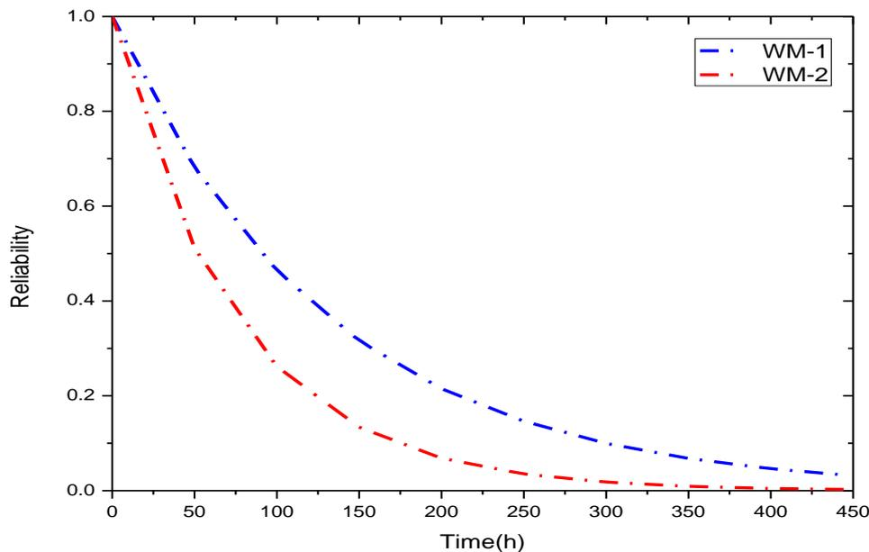
**Figure 3: Comparison of reliability indicators of hydraulic subsystems WM -I and WM**
