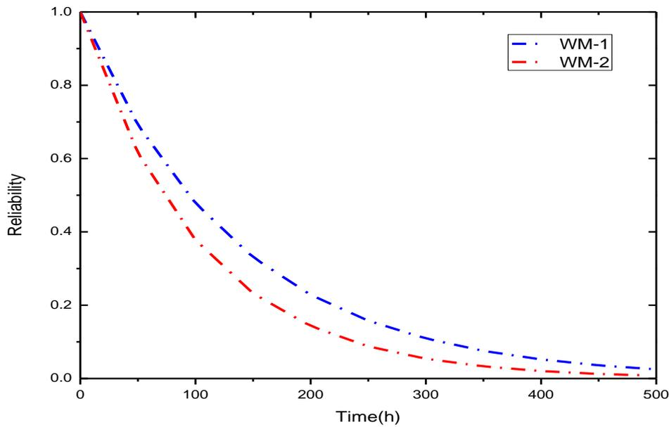
Figure 2: Comparison of reliability indices of WM -I and WM pneumatic subsystems .
