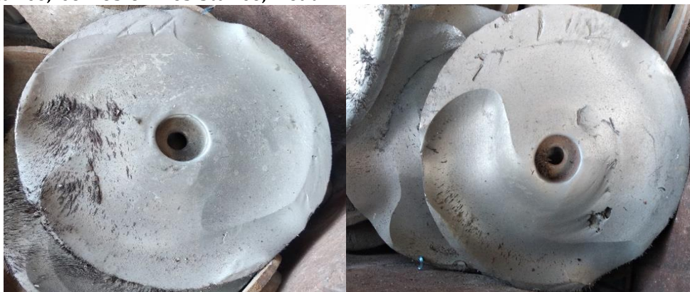
Figure 1. Appearance of a disc cast that has become unusable
