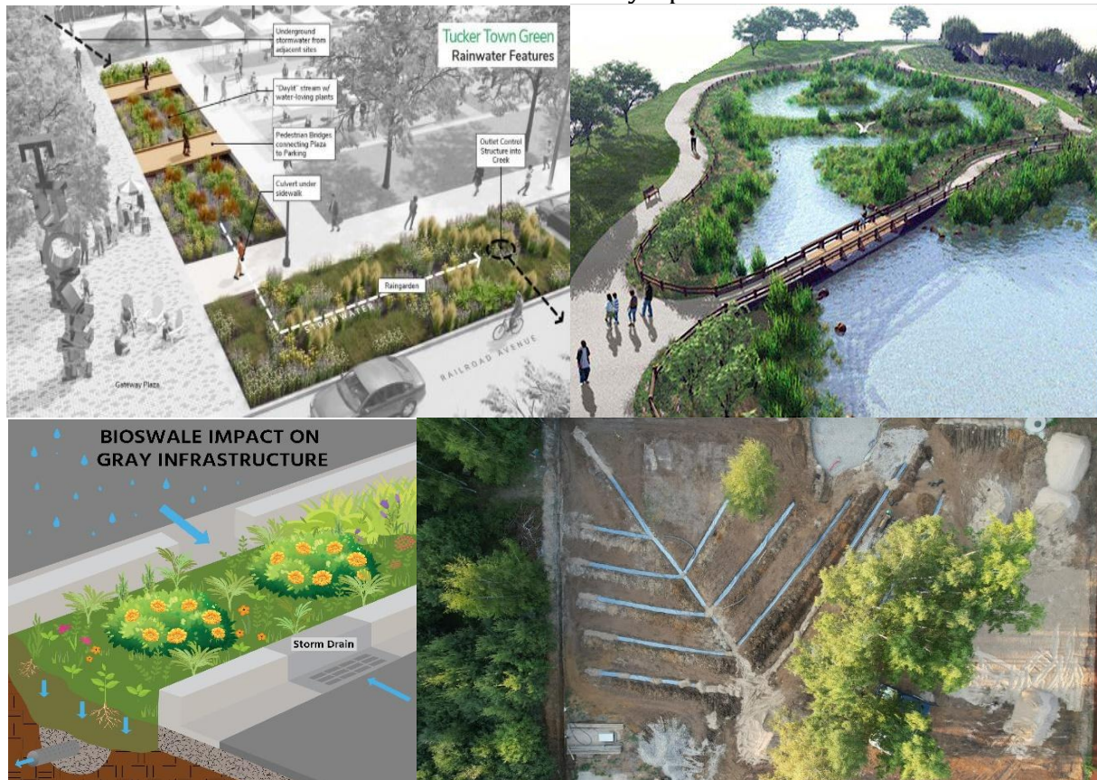
Figure 2. Water and drainage + landscape integration - biofilters, artificial wetlands and green drainage zones
