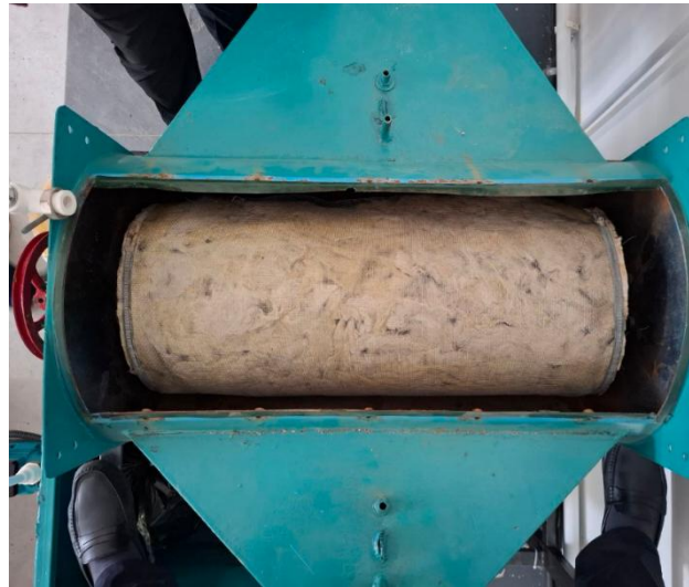
Figure 4. Basalt fiber rotor-filter installed in the apparatus.
