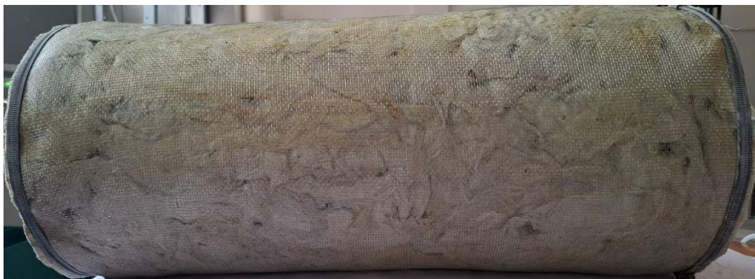
Fig. 3. View of basalt fiber mat rotor filter. (weight of basalt fiber m = 100 grams)
