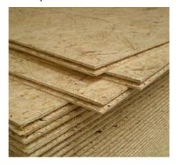
It is characterized by the fact that the collection of chips is carried out in a different direction in each layer. The number of layers in each plate is three or four. Usually, the direction of placement of chips is obtained in the following order:
