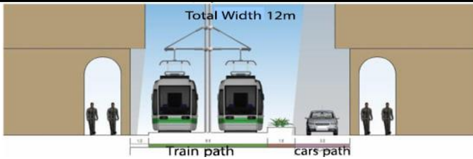
Figure 10. A cross section of the LRT route.
