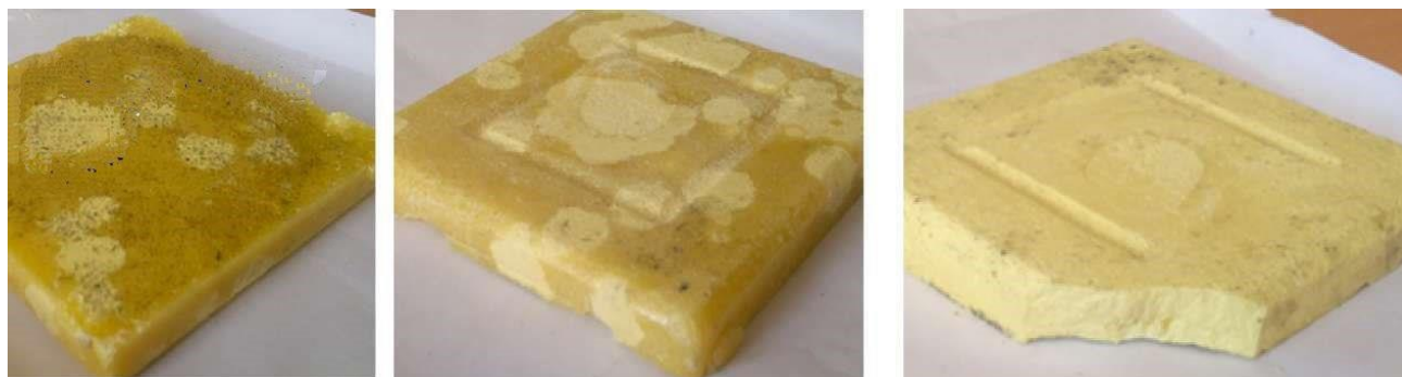
Figure 4 – Sample of initial sulfur after melting and crystallization
