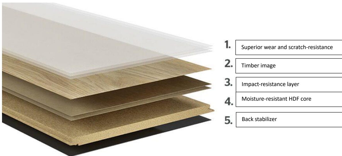
Figure 6: Wood flooring components from Pergo [14].
