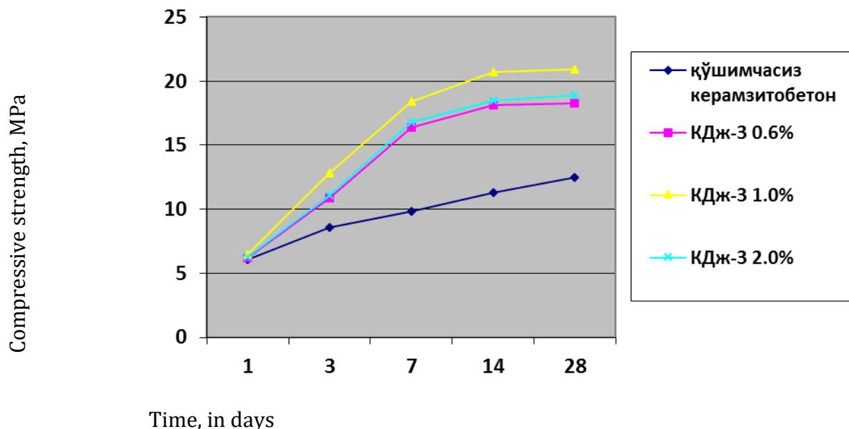
1. compressive strength of expanded clay concrete without additives; 2- 0.6% KDz-3; 3- 1.0% KDj-3; 4 – compressive strength of expanded clay concrete with 2.0% KDz-3 addition compared to cement mass.
