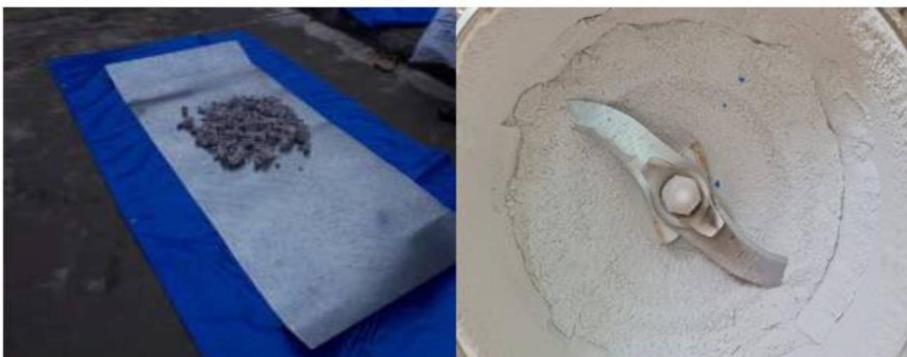
figure (5): Mechanism of crushing the concrete. figure (6): Concrete demolishing waste.
