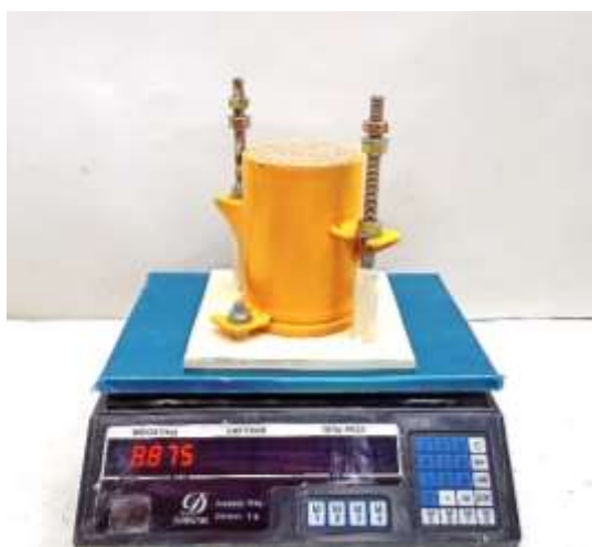
Figure (2) Proctor Test
