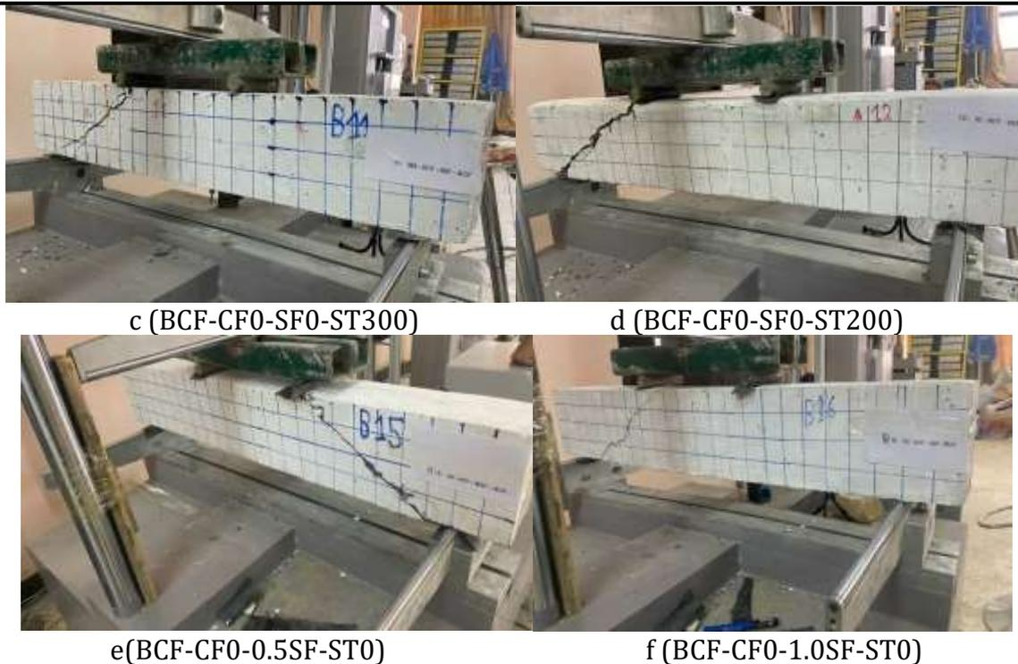
Fig. 9 Failure modes of the test beams as control beam and beams strengthened internally by SFRC or stirrups and without CFRP sheet.
