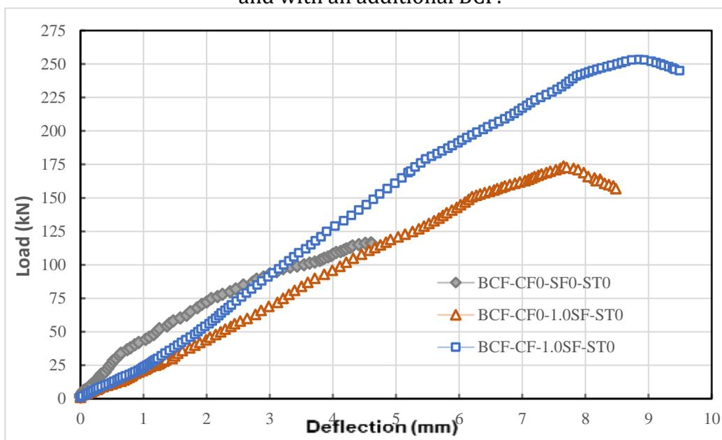
Figure 8. Load-deflection curves for the CB and beams 1.0SF with and without CFRP strengthening and with an additional BCF.
