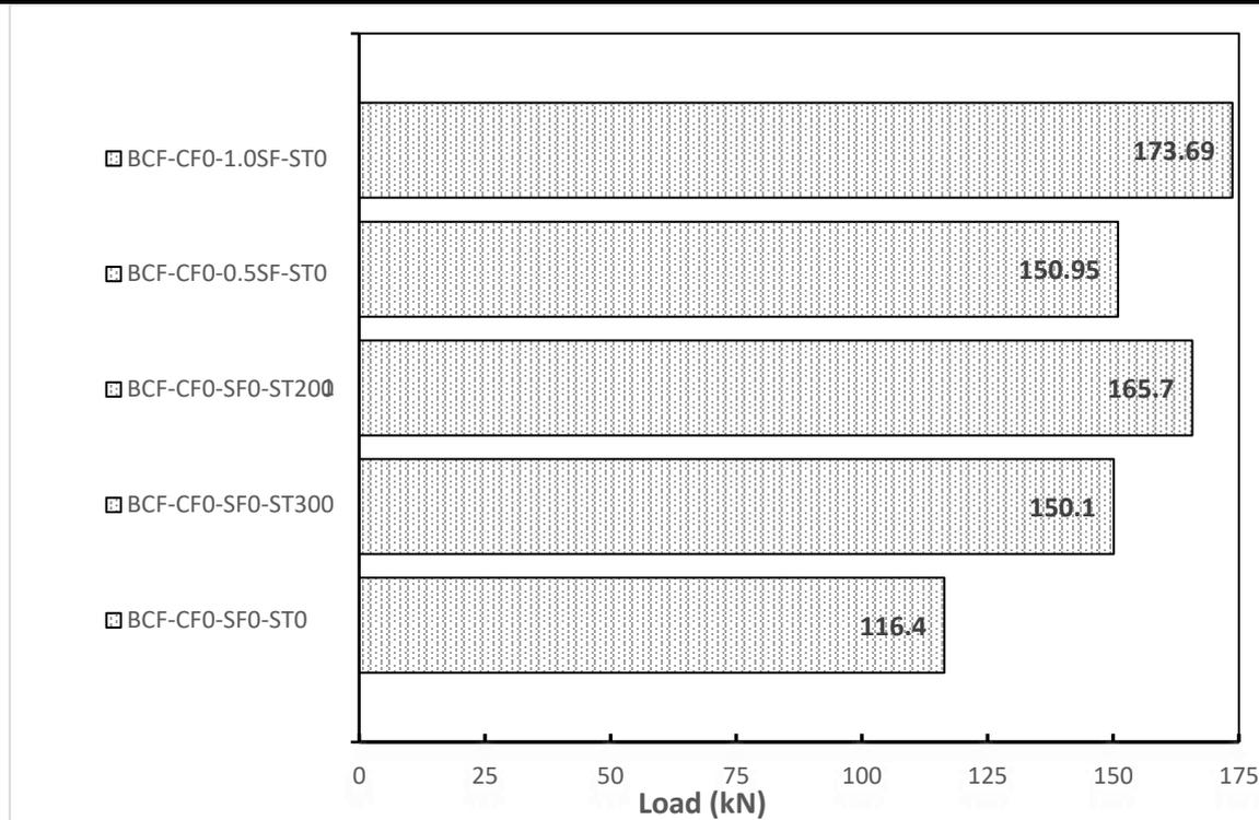
Figure 3 The load-carrying capacity of beam samples with steel stirrups or steel fiber with an additional CFRP Strengthening from the bottom only
