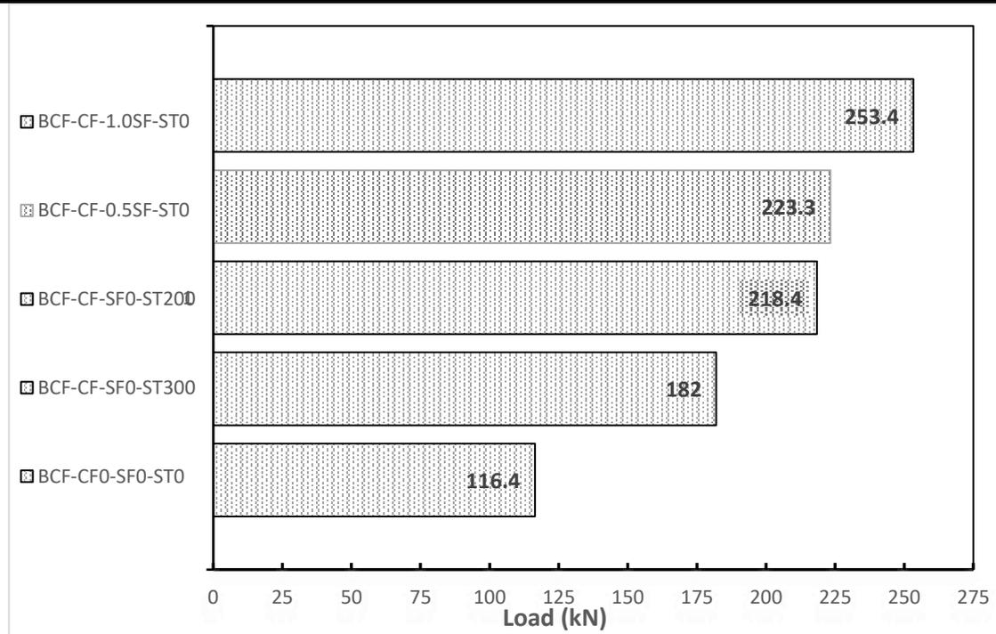
Figure 4. The load-carrying capacity of beam samples with ST or SF with an additional CFRP Strengthening from the sides and bottom.
