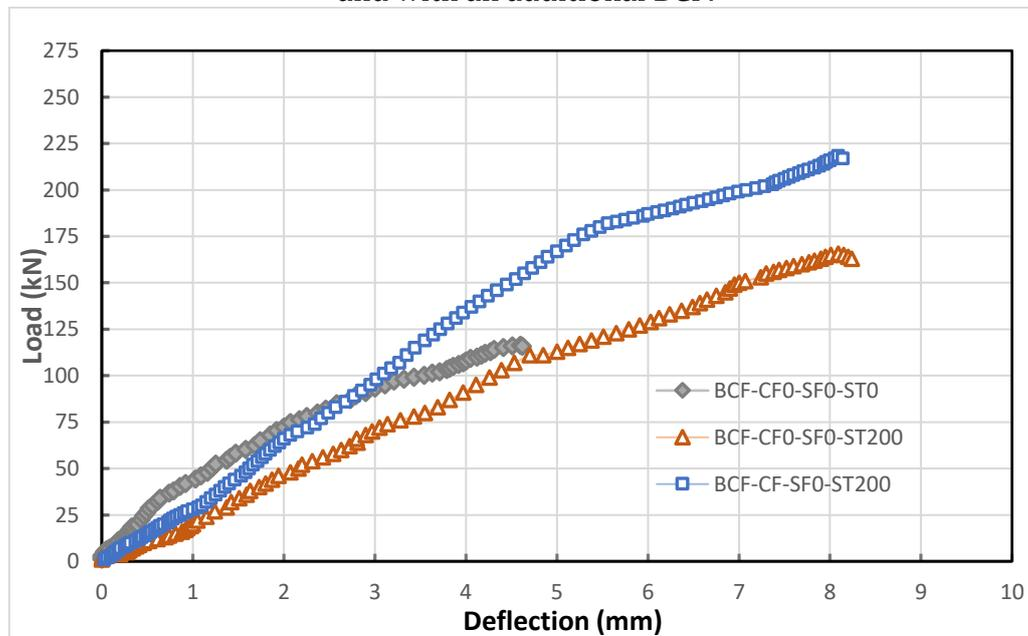
Figure 6. Load-midspan deflection curves for the CB ST200 with and without CFRP strengthening and with an additional BCF.
