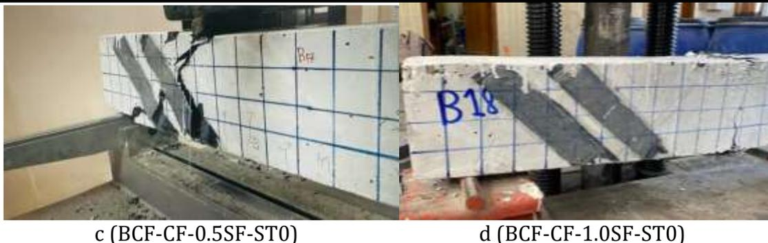
Fig. 10 Failure modes of CB and beams of ST or SF with CFRP addition to BCF
