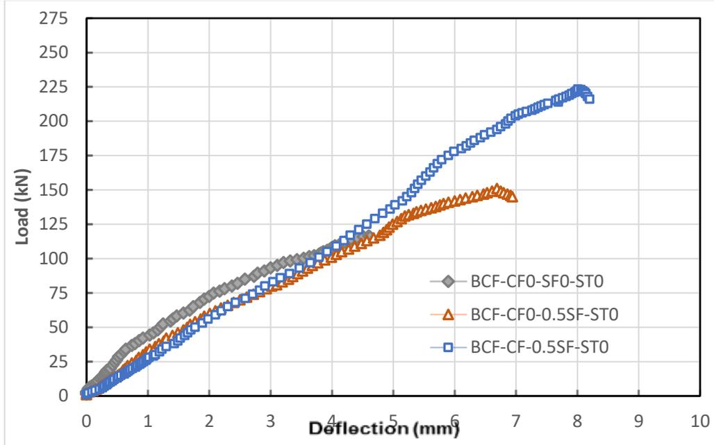
Figure 7. Load-deflection curves for the CB and with beam 0.5SF with and without CFRP strengthening and with an additional BCF.
