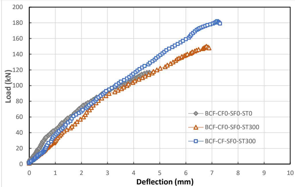
Figure 5. Load-midspan deflection curves for the CB ST300 with and without CFRP strengthening and with an additional BCF.
