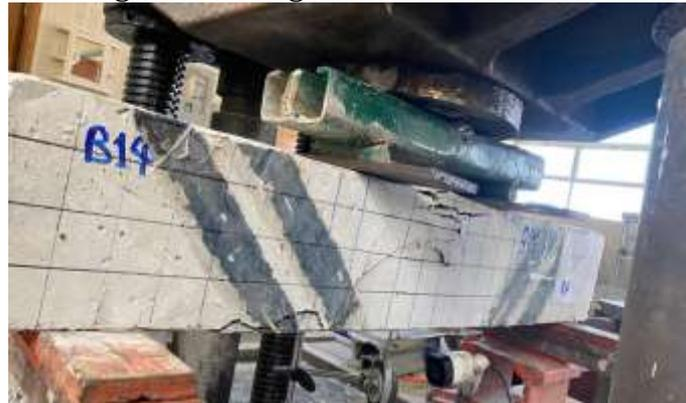
Figure 2. A test beam with inclined CFRP during testing.
