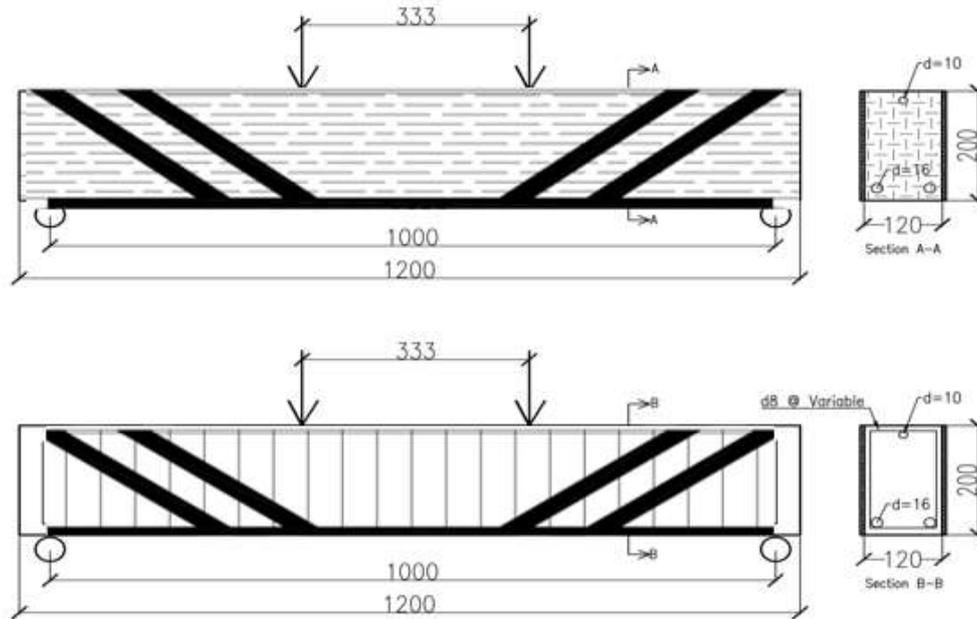
Figure 1. Specimens cross-sections
