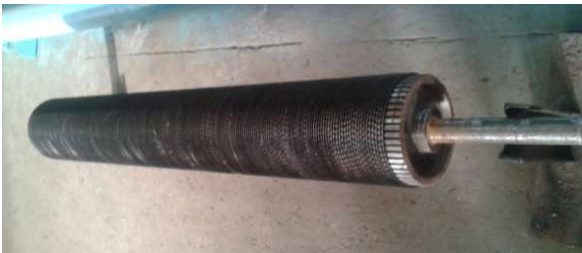
Figure 1. Assembled saw cylinder for 1LB colossal linter.
