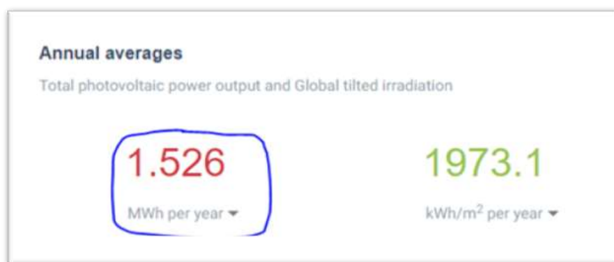
3 Picture. Annual production capacity of a 1 kW photovoltaic system installed on the roof of a building
