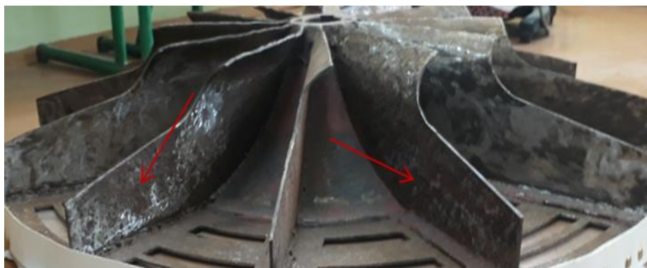
Figure 1. Damage to the working surfaces of the pneumatic transport fan.
