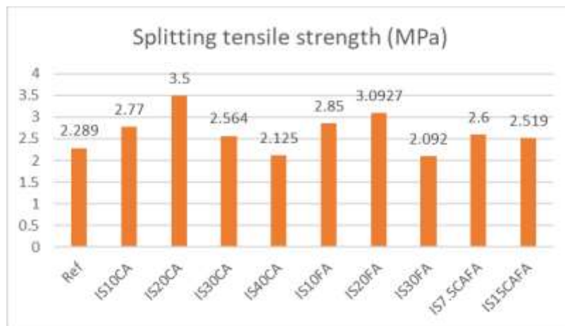
Figure 8. Effect of iron slag on splitting tensile strength
