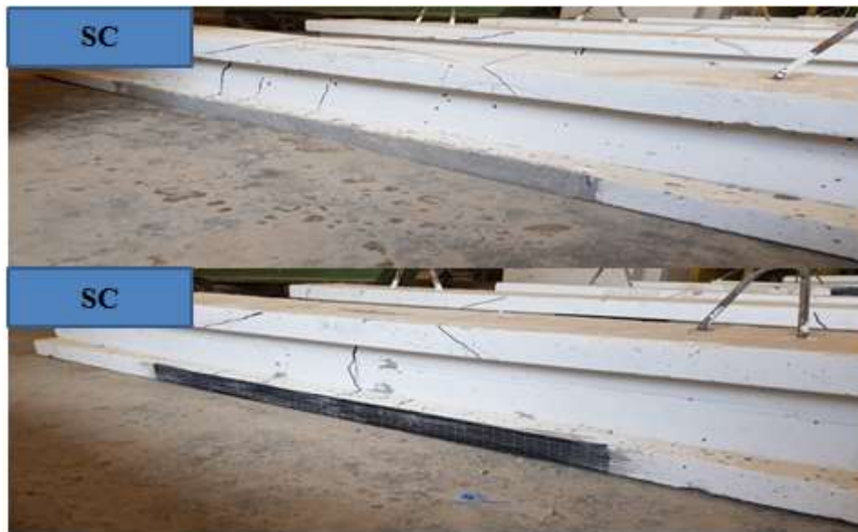
Figure (13) Cracking and failure pattern for SC and SC
