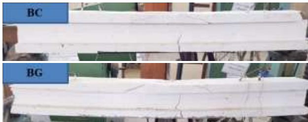
Figure 14. Cracking and failure pattern for BC and BG
