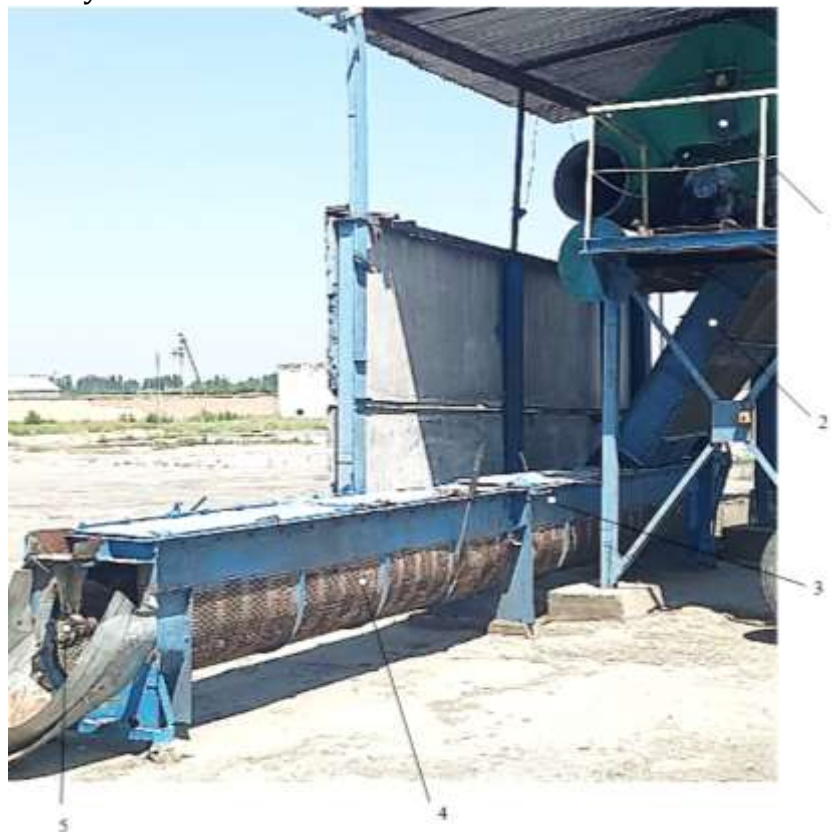
Figure 2. General view of a device for transporting and cleaning cotton from small litter at a cotton gin. 1-cotton separator (SS-15A); 2-patches; 3-conveyor for transporting and cleaning cotton from small litter; 4- mesh surface; 5 pin auger.
