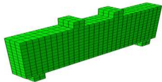
Figure (2-2): for Beam SS-1, the Applied Mesh.
