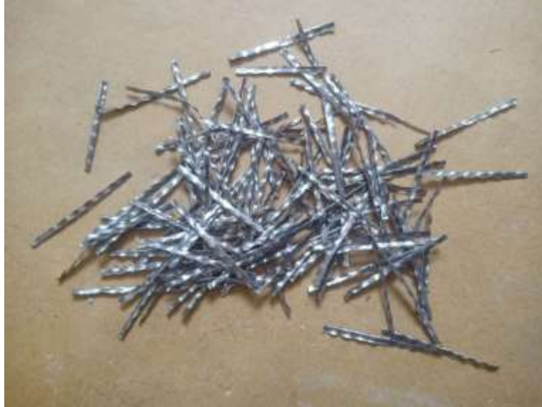
Figure (1): Crimped steel fiber used
