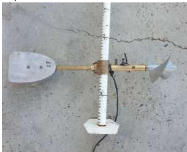
Rice. Fig. 3. General view of the hydrometric meter GR-21-M1
