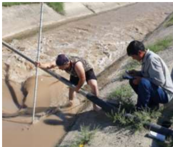
Rice. 4. The process of measuring the flow rate of water using a hydrometer vane
