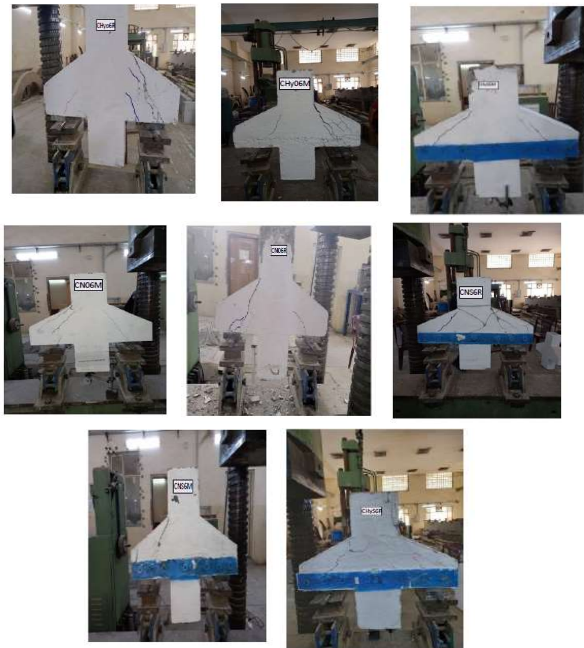
Figure 4. Cracks patterns of corbels after testing.
