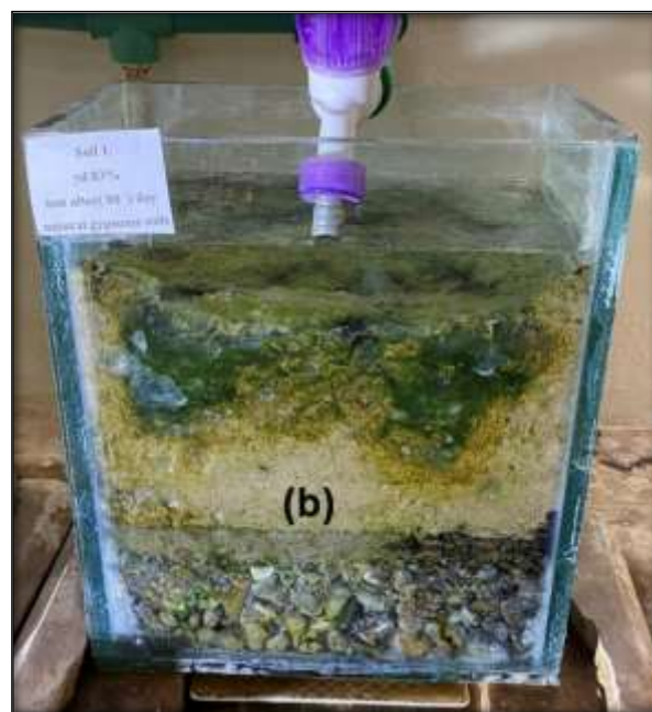
Plate 6: The model's test after 80 (days) (a) PPF-treated gypsum soil: (b) natural gypsum soil
