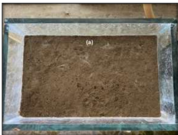
Plate 4: The model's test after 22 (days) (a) PPF-treated gypsum soil: (b) natural gypsum soil
