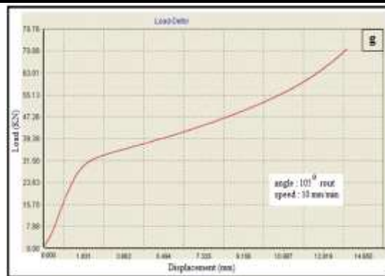
Fig.8 : Load – Displacement relationship of compression test for specimens according to the angle of die and speed of punch
