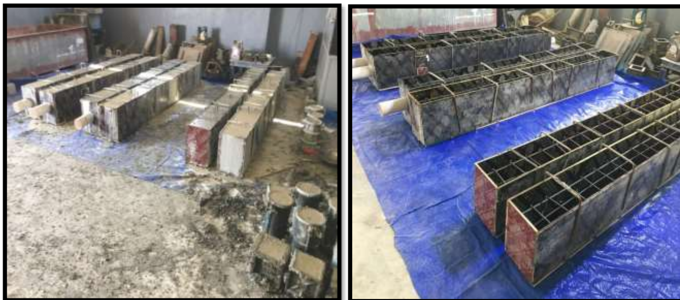
Figure 2: Molds and reinforcement steel used for casting sample
