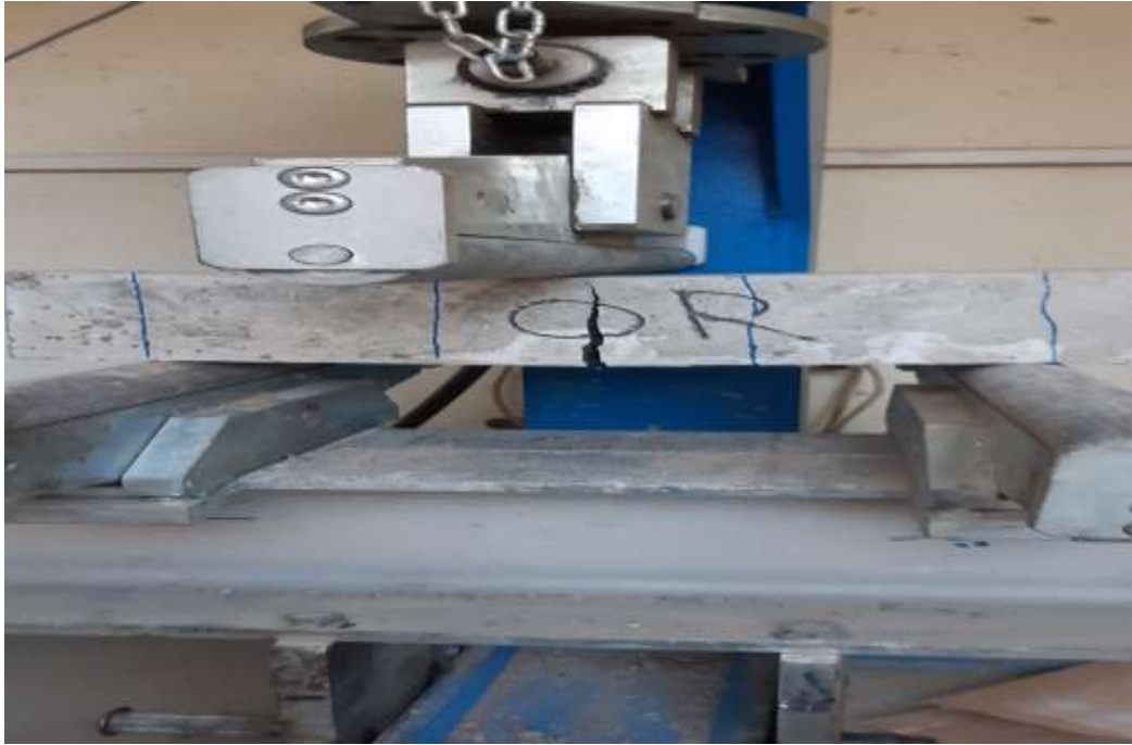
Figure 2.2 Fracture initiates of the examined beams
