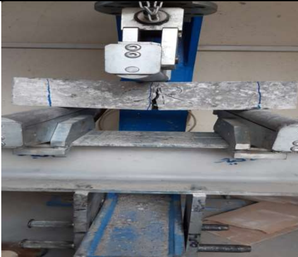
Figure 3.3 Failure mode of plain GHPC beams
