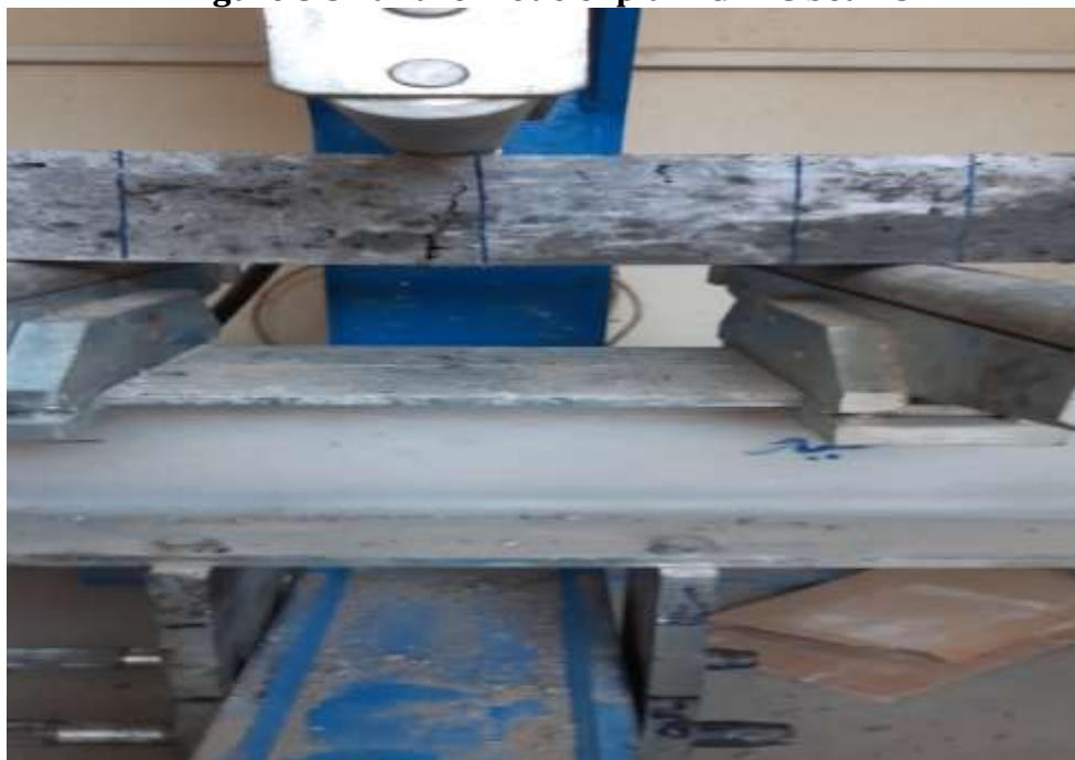
Figure 3.4 Failure mode of carbon fiber reinforced GHPC beams
